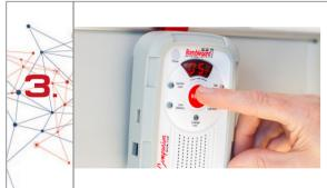
To deactivate SLEEP mode hold RESET button until LCD shows 'ON'
