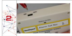
Switch transmitter 'ON'
